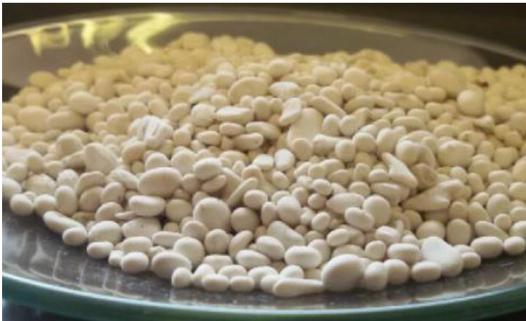
Phosphorus recovered as struvite (Source: GENOCOV research group, Universitat Autònoma de Barcelona, http://www.genocov.com )
