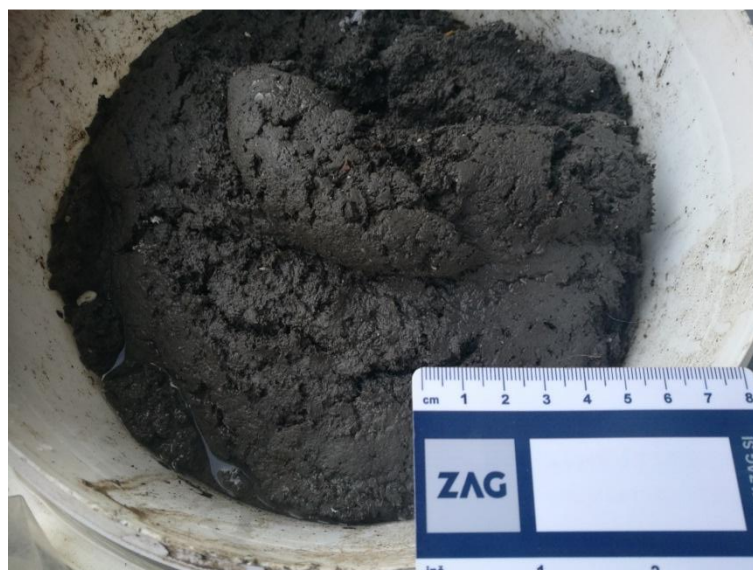
Figure 25: Sewage sludge mechanically dehydrated and hygienized with lime and prepared for laboratory testing
